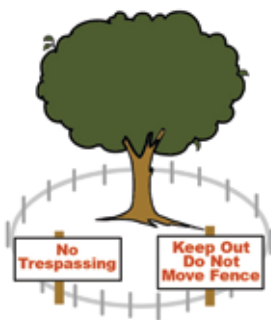
Figure 5a. Placing a protective fence around the critical root area assures tree survival.
